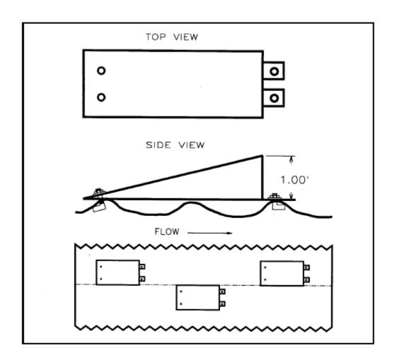
Figure VII-47. Corrugated metal pipe steel ramp baffles.
