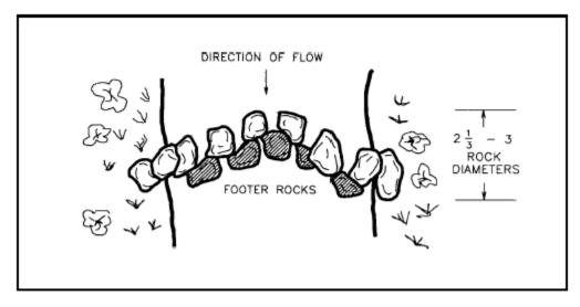
Figure VII-23. Vortex boulder weir, plan view (Rosgen, 1993).
