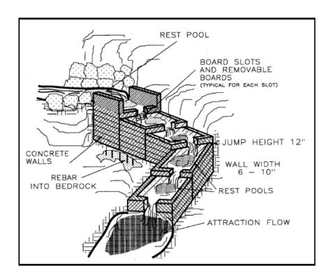
Figure VII-39. Step-and-pool fishway.
