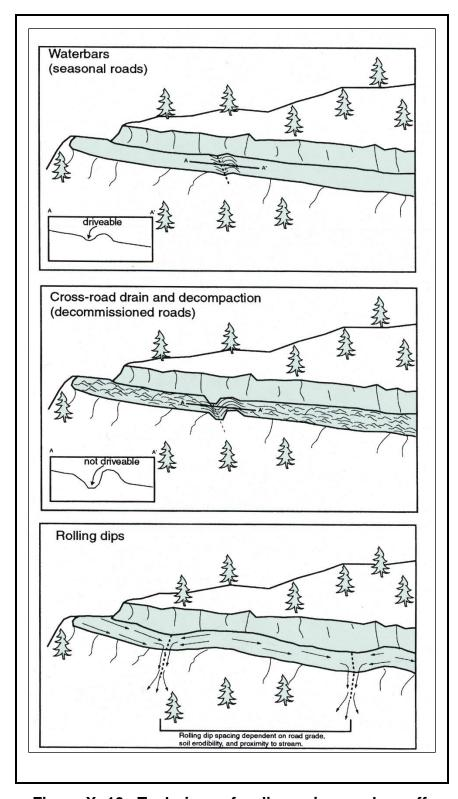
Figure X- 10. Techniques for dispersing road runoff.
