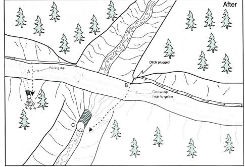
Figure X- 13. Typical upgraded stream crossing.
