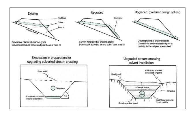
Figure X- 14. Typical culvert installation on non fish-bearing streams.
