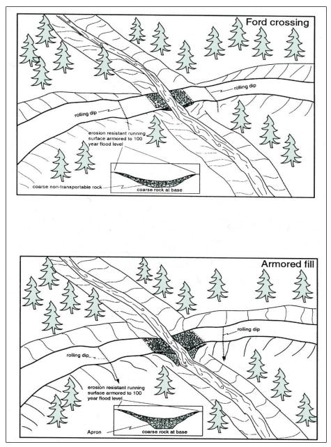
Figure X-15. Typical armored fill stream crossing.
