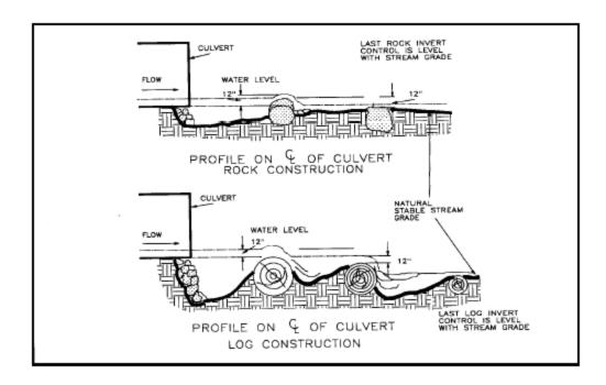
Figure VII-42. Back-flooding weirs.
