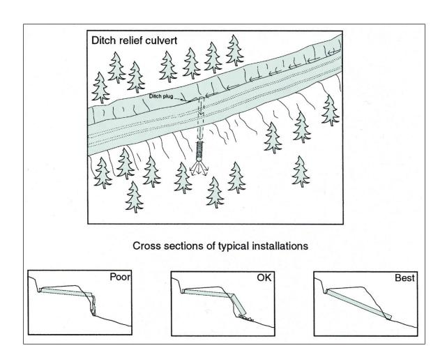
Figure X- 20. Typical ditch relief culvert installation.
