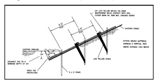
Figure VII-60. Brusch Mattress Cross Section (L. Prunuske, 1997)
