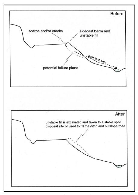
Figure X- 17. Removal of unstable sidecast materials.
