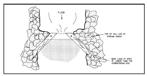
Figure VII-31. Upstream-V log weir with a low-flow notch.
