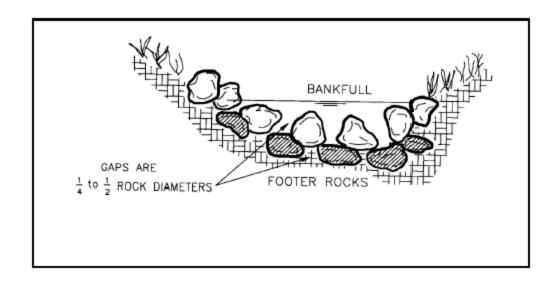
Figure VII-22. Vortex boulder weir, cross section view (Rosgen, 1993).
