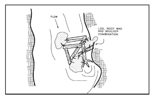
Figure VII-20. Log, root wad, and boulder combination.
