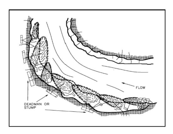
Figure VII-54. Tree revetment.
