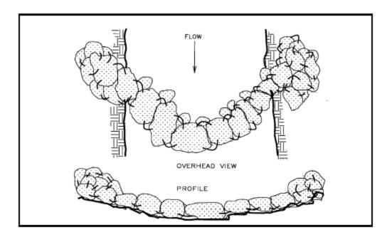
Figure VII-21. Downstream-V boulder weir.
