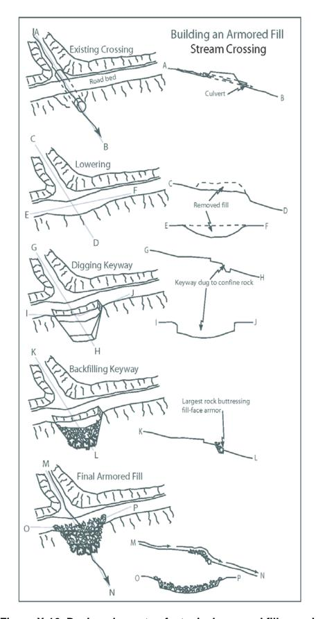
Figure X-16. Design elements of a typical armored fill crossing.
