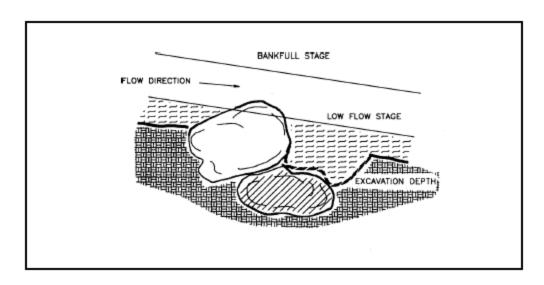
Figure VII-24. Vortex boulder weir, profile view (Rosgen, 1993).
