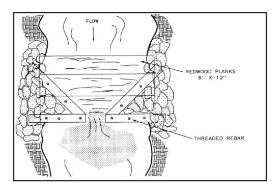
Figure VII-33. Log constrictors over planks.
