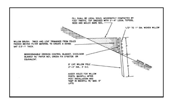
Figure VII-58. Willow Wall Revetment (L. Prunuske, 1997)
