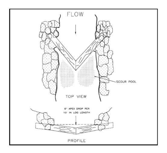
Figure VII-28. Downstream-V log weir.
