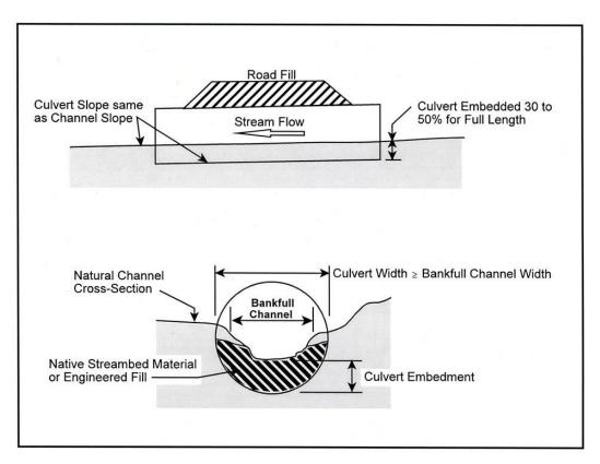
Figure IX-A- 2 Stream simulation design option.
