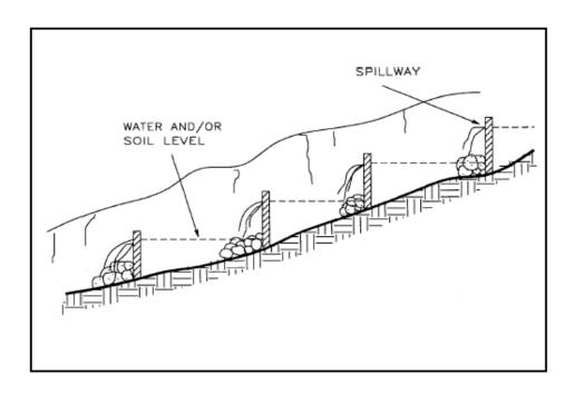
Figure VII-67. Checkdam placement. (Prunuske, 1987).
