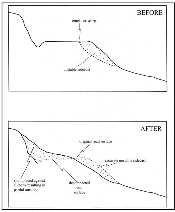
Figure X- 11. Partial outsloping for road decommissioning.
