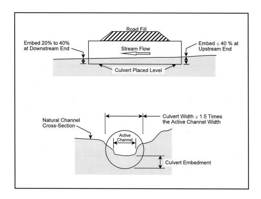
Figure IX-A-1. Active channel design option.
