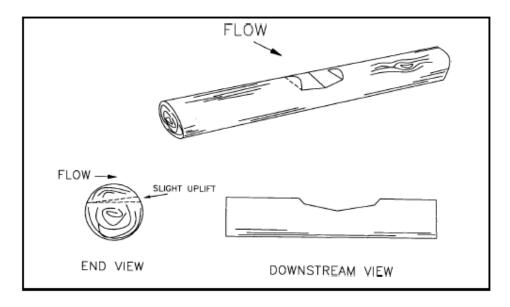
Figure VII-27. Straight log weir with low-flow notch.
