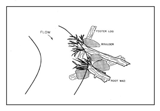
Figure VII-55. Plan view of native material revetment (Rosgen, 1993)
